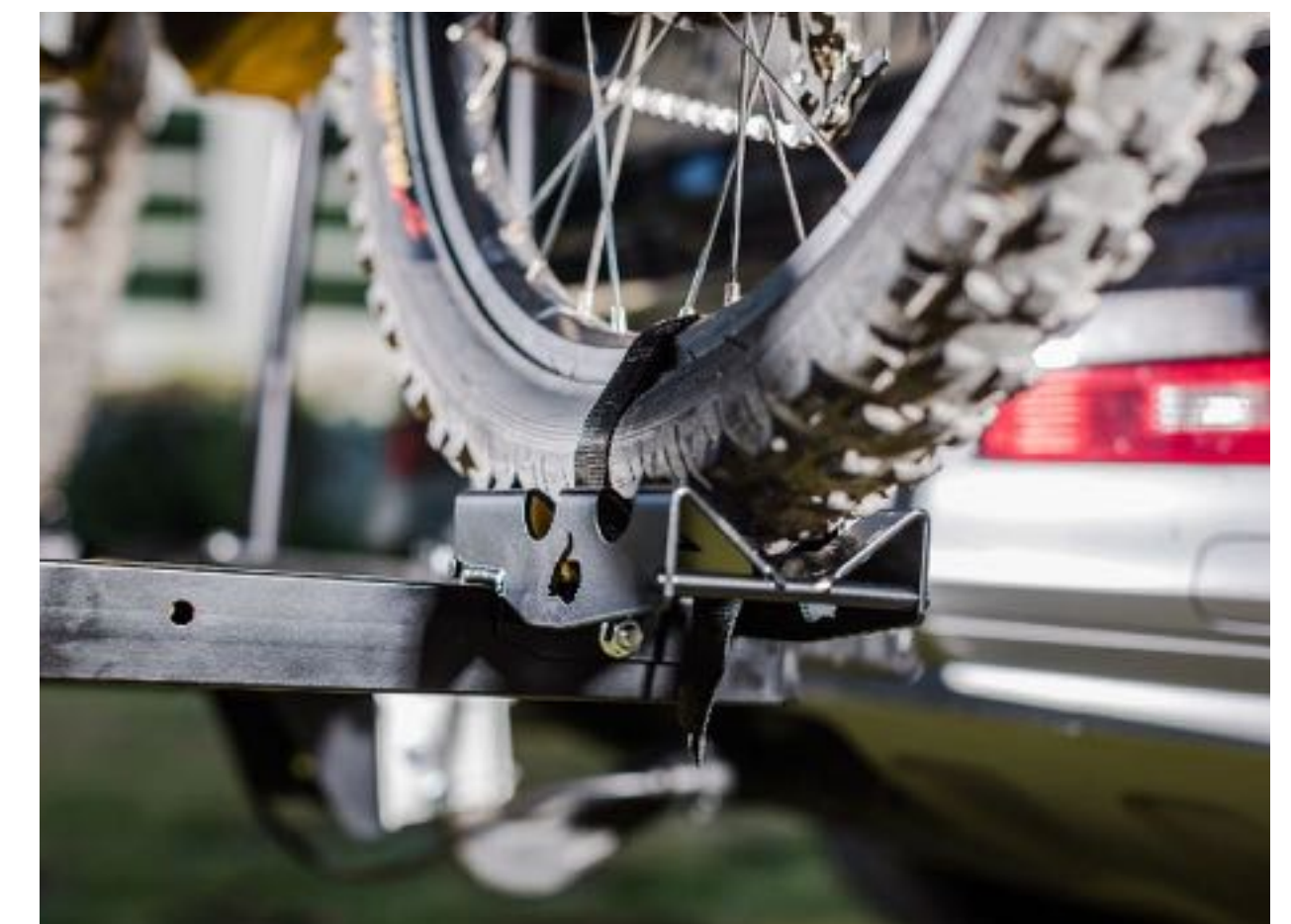
Support and strap for wheel
