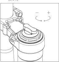
Main air chamber Fill in the air according to suggested pressure meter.
